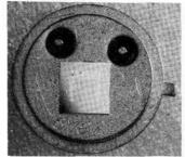
NEW PHOTODIODE (above) is exceptionally resistant to effects of ionizing radiation. The diode itself (the squared horseshoe portion of the device) is actually only 1 mm (0.0040 inch) across. Two of the device developers are (left) Russ Keefe and project coordinator Jamie Wiczer (both 1142).
